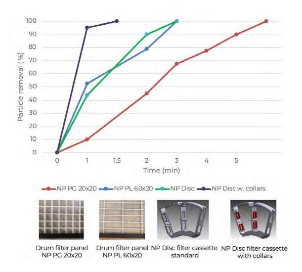
Figure 3: Comparison of how quickly different filter panels and cassettes are lifting out 100 ml of feed pellets with a diameter of 5 mm.
