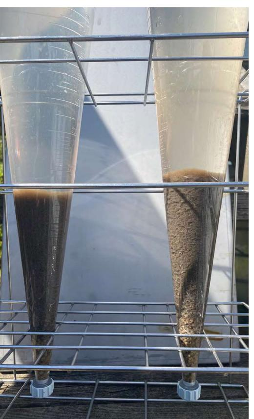
Sedimentation of reject water from a disc filter, left, and a drum filter, right, showing that there are more dissolved fines in the latter.
